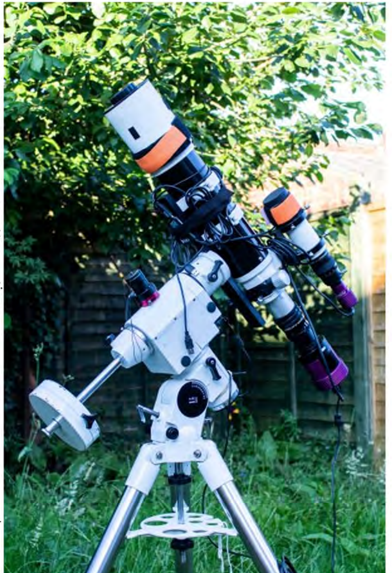
Using an APS-C Camera and a 0.8x Reducer You Can Fit Large Targets In Frame. FoV Emulator from Stellarium
