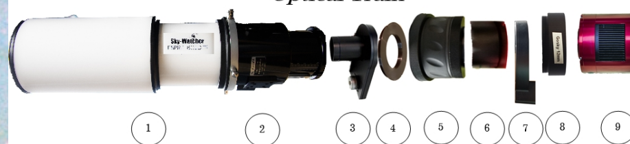
Skywatcher Esprit 80 APO with ZWO Monochrome Optical Train
