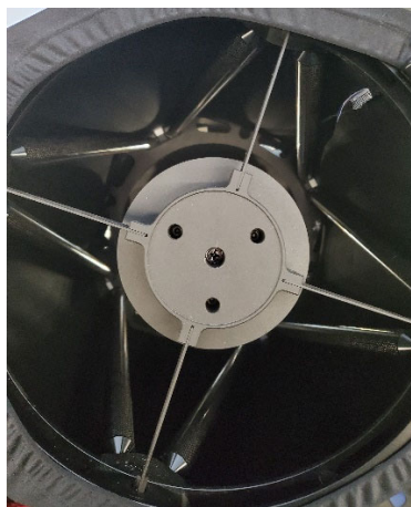
Astro-Tech 14" RC reflector telescope with secondary mirror and supports
